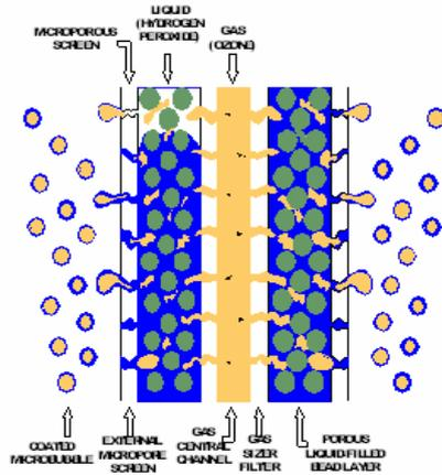
The reaction of ozone with the contamination forms hydroperoxides, which in turn creates additional OH radicals. This double formation of OH radicals ensures a very high oxidation capacity.
